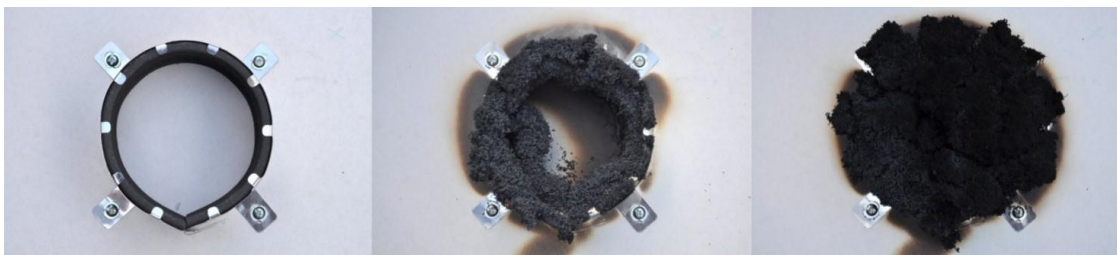
Figure 5 -The operation of a fire collar with intumescent material
